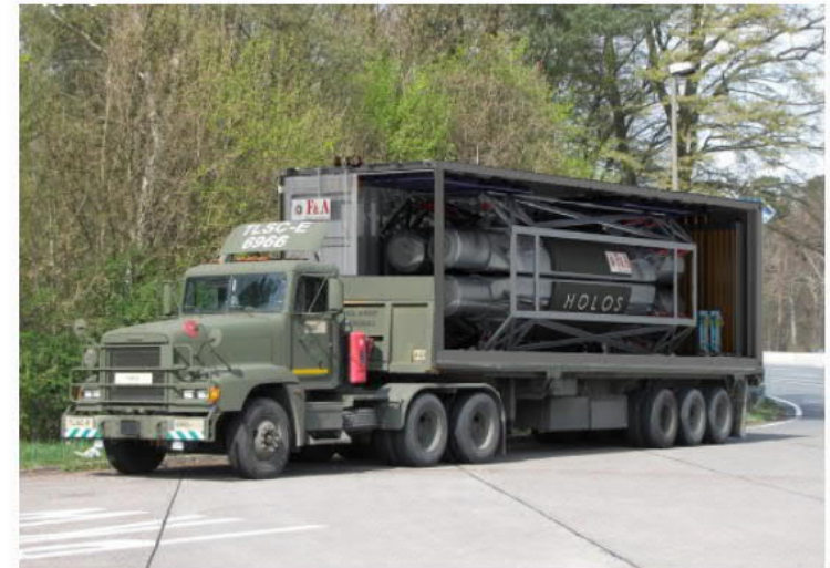
A U.S. Army Truck hauling a Holos small nuclear generator with skin, shields and auxiliary ... [+] HOLOS
